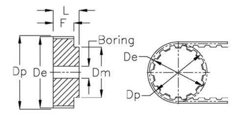
Type = AT10Belt width = - 25 mm Weight = 1.516 = 150.95De Dm = 95 = 76.4Dp F = 30 L = 40 Pre-drilled = 16
